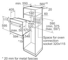
measurements in mm
