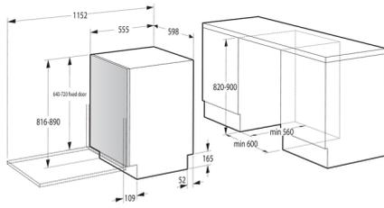
Fixed door height 2L, 645-729 (mm), Sliding door 688-768 (mm)
